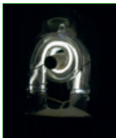
Picture 3: As the resistance drops, the tube fills up with xenon, which is now in a plasma state.
