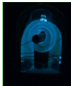
Picture 4: The full current now flows through the tube and radiates light.
