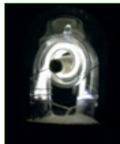
Picture 2: The capacitor lets the current charge flow through the tube which causes a reaction with the xenon gas.
