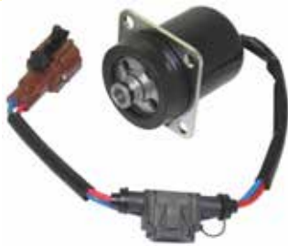
Injector assy - LPG REF 136TA3088 - K15 (2003/07- ) REF 136TA3089 - K21 (2003/07- 2007/08 ) REF 136TA3090 - K21 (2007/09 - ) REF 136TA3091 - K25 (2003/07- 2007/08 ) REF 136TA3092 - K25 (2007/09 - )
